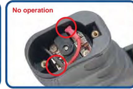
Check the wire set contact with motor.
