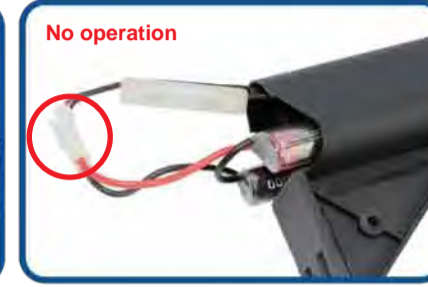
Check the battery and connector.
